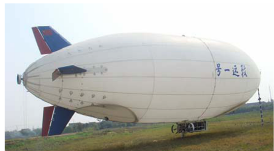
Fig. 1 Remote and autonomous control fuel-cell-powered ZHIYUAN-1 airship.
